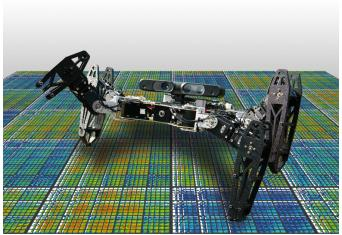
**Figure 6. Six-legged robot.** The robot uses the results of offline, simulated evolution to adapt quickly to a variety of damage conditions, such as a broken leg. Each point on the colored floor represents a different type of gait, i.e. a gait that uses the robot's legs in different proportions. The assumption was that that the cell in this map that required the robot to walk without using any of its legs would be impossible to fill. But, to the researchers' surprise, evolution found a way.
