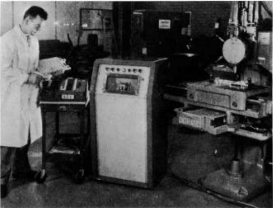
The ECS Digimatic control system, advertised as “numerical control for the small shop.” From The Tool and Manufacturing Engineer , November 1, 1960.
