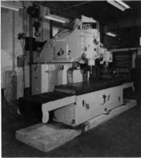
Air Force Cincinnati Hydrotel vertical milling machine, before being converted to numerical control. Massachusetts Institute of Technology Archives.
