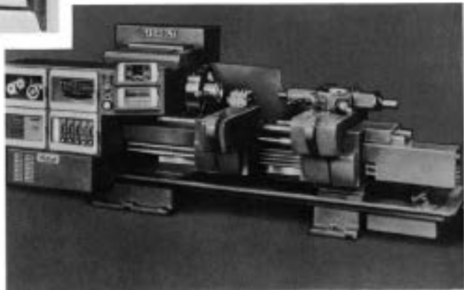
Gisholt Factrol lathe with record-playback control system conceived by Leif Eric de Neergaard. From Gisholt Machine Company brochure, courtesy of L. A. Leifer.
