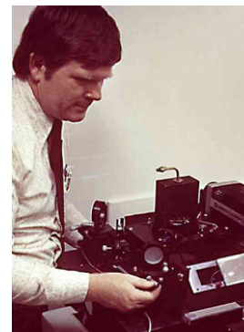
Gary Starkweather ca 1971 at PARC, and his hand-built first laser printer (500 pixels/inch and 1 page/second)
